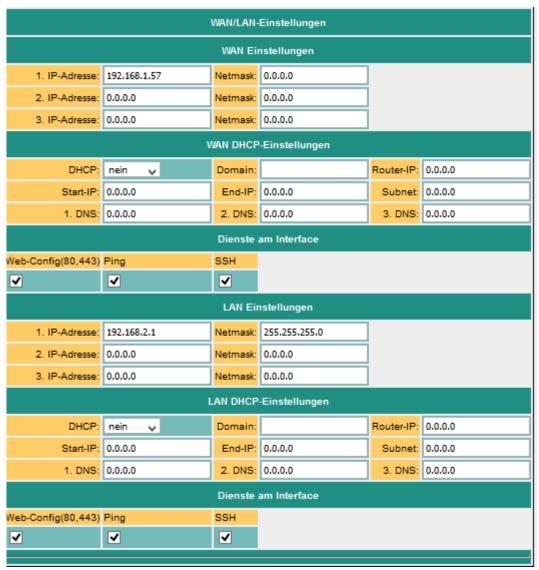
The WAN/LAN port can each receive up to 3 different IP addresses and subnets.
