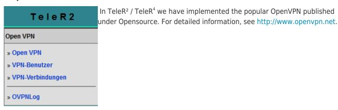
Here I would briefly explain the function of the OpenVPN, as implemented in the TeleR<sup>2</sup> / TeleR<sup>4</sup> Basically there are two operating modes of the OpenVPN: server or client. The device is normally configured as a server on the plant (machines).
