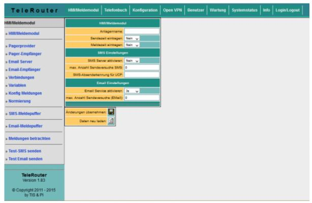
With the HMI-Notification Module SMS and email messages (error and maintenance messages) can be, depending on the event, sent automatically to practically any number of recipients. The system automatically assigns the messages to the respective recipients and sends the message via the correct provider.
