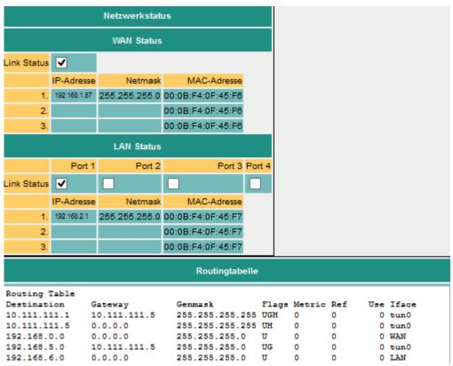
Displays all currently assigned IP addresses and link states of the individual ports. You can also find the current routes.
