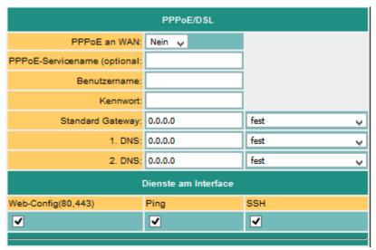
Set the parameters for operation on a DSL/cable modem here. For the overview and for the easier configuration, the settings for standard gateway and DNS can be set here. As a rule, this should be set to "auto from PPPoE".
