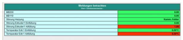
In the menu item **View messages** you can view the current status of the messages. All message states of the configured messages are displayed there. So also these, which can not generate SMS. As a result, a state can be obtained via the system without PLC programming software. The message window is updated every 3 seconds. Red fields indicate that there is a violation of the limit value. Google Übersetzer für Unternehmen:Translator ToolkitWebsite-Übersetzer
