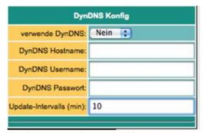
If TeleRouter to be reached by OpenVPN as via the Internet, the Internet IP address of the device must be known. Meaningful here is not to work with a fixed IP address because the provider possibly allocate a new IP address here after new connection establishment (eg via PPPoE). It makes more sense here to access the device always with the same domain name.
