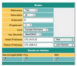
Here the modem parameters are defined. A modem connection is realized as a PPP connection. This allows also be used with TeleRouter alia dial routers. An ideal replacement for example is TeleService IE from Siemens. In the bottom line can be determined which services are available at the interface.
