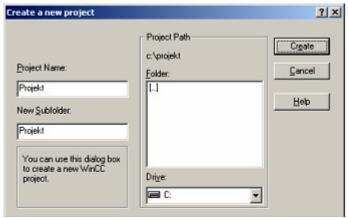
4. OK" leads you to a new dialog. Type in the "Project Name" and the "Subfolder" of the "Project Path" With "Create" the chosen configuration is confirmed.
