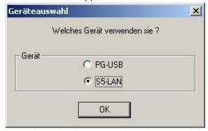
3. Device selection Now select the type of device. Select "S5-LAN + + / PG-USB-cable / USB-RS232-converter" and confirm with "OK".
