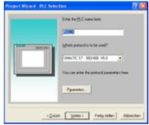
4. "Next" leads you to a new dialog. Type in the specfic fields the name of the PLC device and choose the used PLC in the driver selection
