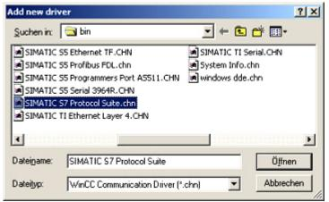
7. In the dialog "Add new driver" select the driver which fits to your PLC For a S5 PLC, you can choose the file SIMATIC S5 Programmers Port AS511.chn. If you are using a different PLC please inform yourself which driver fits with your PLC.
