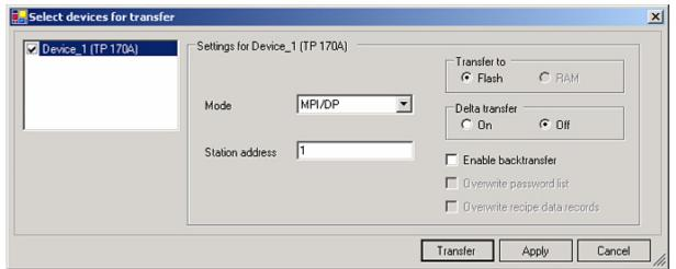
9. Press the button "Transfer" to start communication with the terminal. Your project is about to be transferred. The communication with the operator terminal is so successfully established .
