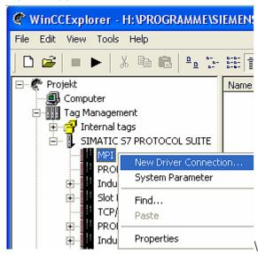
6. For a proper working communication with the PLC there must be defined how the software has to communicate with the PLC Therefore right click on "Tag Management" to open the context menu. Choose "Add New Driver ...".
